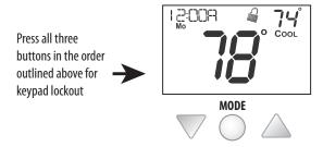
To *unlock* the keypad, press and hold the MODE button. While holding the MODE button, press the WARMER and COOLER buttons together.
