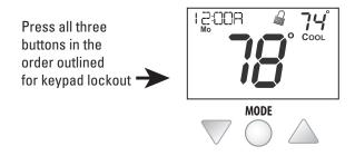
To **unlock** the keypad, press and hold the MODE button. While holding the MODE button, press the WARMER and COOLER buttons together, for two seconds. The icon will disappear from the display, then release the buttons.
