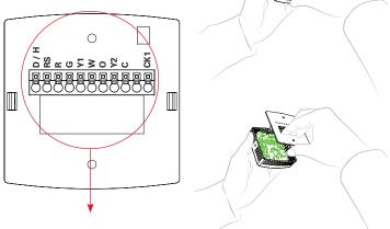
IMPORTANT: This thermostat requires both R (24 VAC Return) and C (24 VAC Common) wires be connected to the backplate terminals to operate properly.
