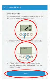
4. Press the fan button for 5 seconds, then press the cooler/down button to put the thermostat in "AP MODE", then return to the app and select "Next".
