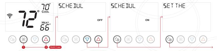
Press and hold the fan and warmer (up) buttons for 2 seconds to enter schedule mode for programming a schedule. While in schedule mode, press the mode button to advance through each setting for each day of the week and each time period of each day. To exit schedule mode and return to the home screen at any time, press and hold the mode button for 2 seconds. The system will return to the home screen automatically after 2 minutes of inactivity.
