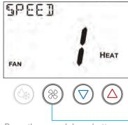
Press the up and down buttons to cycles through available auto speeds 1–5.
