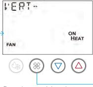
Press the up and down buttons to toggle the heat mode vertical swing off and on.
