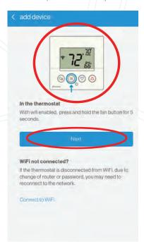
3. Press and hold the fan button on the thermostat for 5 seconds to put the thermostat in "Wireless Setup" mode, then select "Next" in the app.
