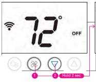
Press and hold the fan and cooler (down) buttons to enter the settings for Away mode.
