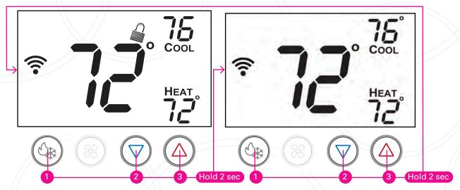
To disable, or "lock" the keypad, press and hold the mode button. While holding the mode button, press the warmer (up) and cooler (down) buttons together, for two seconds. The lock icon will appear on the display, then release the buttons.
