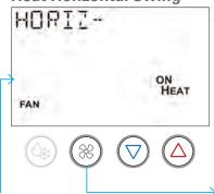
Press the up or down buttons to toggle the heat mode horizontal swing off and on.
