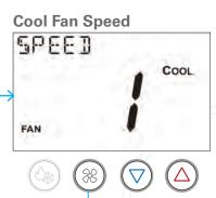
Press the up and down buttons to cycle through the available fan speeds of auto and 1 (low) through 5 (high). 1–5.
