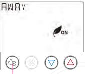
Press the warmer (up) and cooler (down) buttons toggles away on or off.
