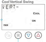
Press the up and down buttons to toggle the cool mode vertical swing off and on
