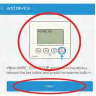
4. Press the up/warmer button on the thermostat to display the 6-digit pairing code, then return to the app and select "Next".
