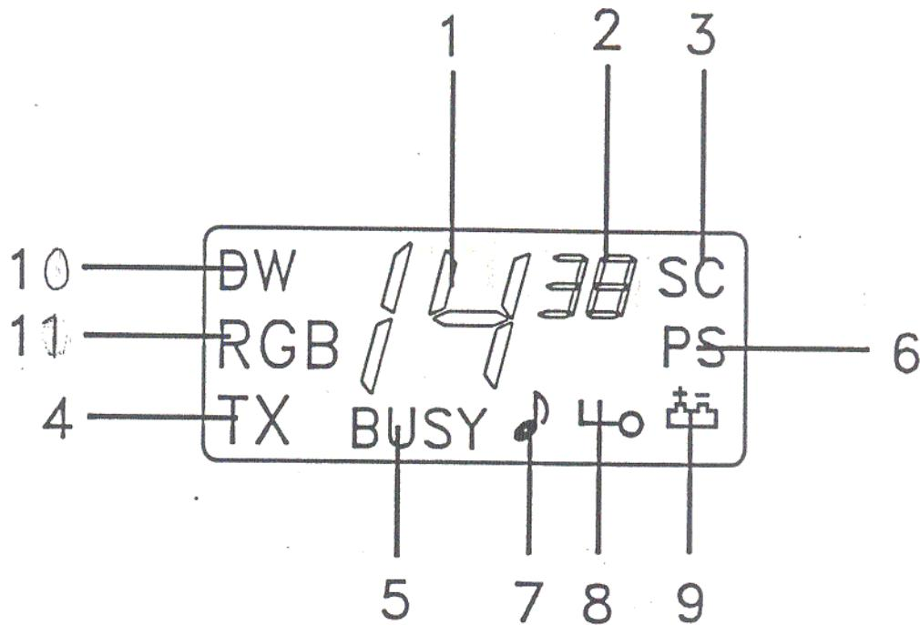
The KF-2200 is equipped with an LCD display to indicate its settings and functions. The Display incorporates automatic backlighting to allow it to be seen in the dark. Pressing any of the buttons except the PTT (Push-to-Talk) button, will illuminate the display. The display will remain lit for 5 seconds after any of these buttons is pressed.
