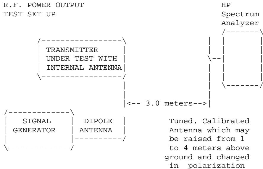
Equipment placed 1 meter above ground
