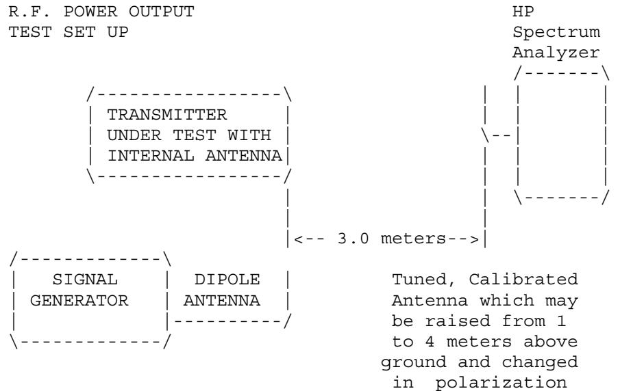
Equipment placed 1 meter above ground
