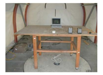
Conducted Emission Test Setup – Rear View
