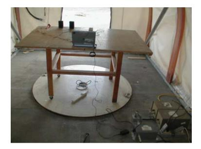
Radiated Emission Test Setup – Front View
