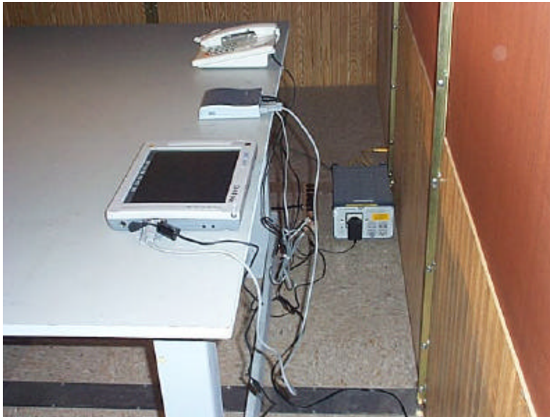
Conducted Emission Setup, showing cable placement
