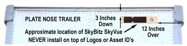
For a Sheet and Post Nose Trailer, the SkyVue will be mounted to the front wall in relatively the same orientation and location unless the location and spacing of the rivets and posts on the front wall prohibit fitting the SkyVue horizontally as described. In some instances, the SkyVue will need to be mounted vertically about 3 inches down from the bottom of the top rail, and about 12 inches from the roadside edge with the connector at the top as shown below.
