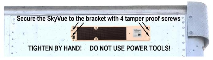
Using a hand driver, secure the SkyVue to the bracket with four, 10-32 tamper proof screws
