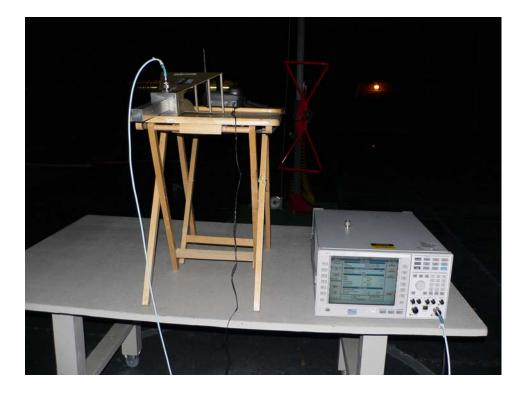
**TX Radiated Emission - Rear View**
