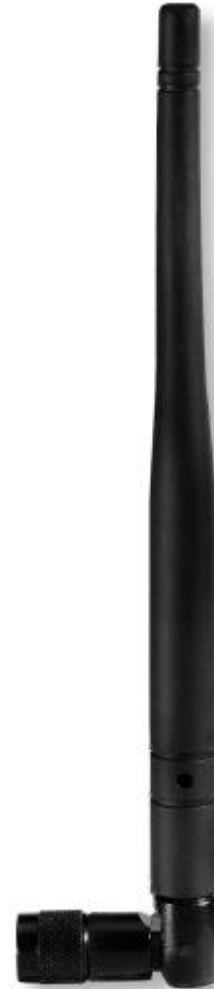
Centerfed 1/2 wave dipole antenna.
