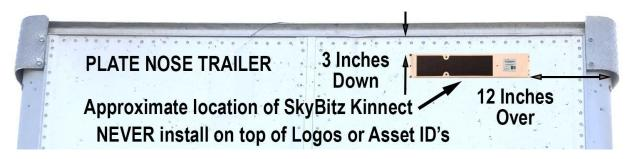
For a Sheet and Post Nose Trailer, the Kinnect will be mounted to the front wall in relatively the same orientation and location unless the location and spacing of the rivets and posts on the front wall prohibit fitting the Kinnect horizontally as described. In some instances, the Kinnect will need to be mounted vertically about 3 inches down from the bottom of the top rail, and about 12 inches from the roadside edge with the connector at the top as shown below.
