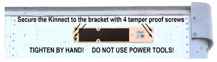
• Using a hand driver, secure the Kinnect to the bracket with four, 10-32 tamper proof screws
