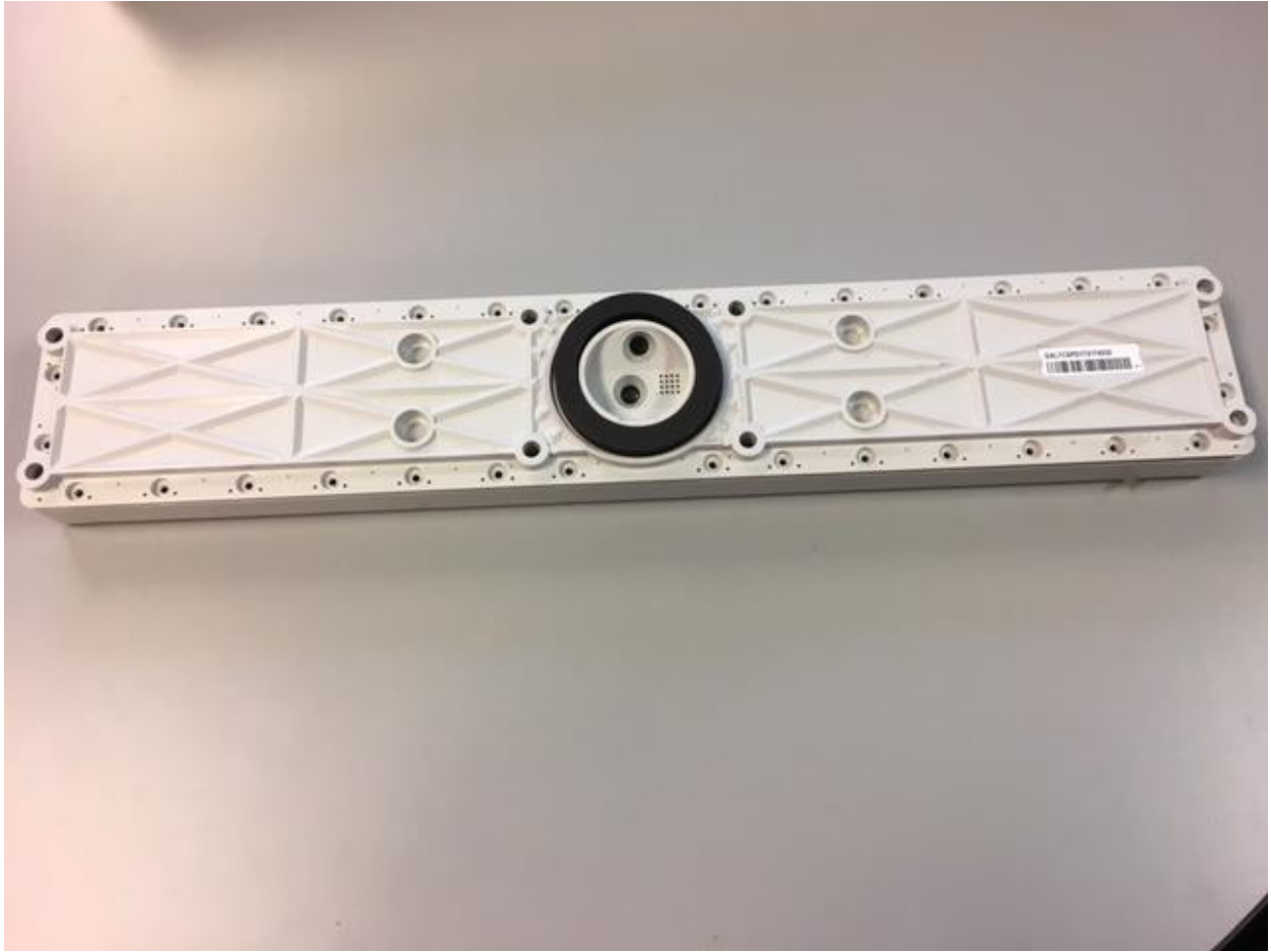
BOTTOM/INTERNAL SIDE OF UNIT WITH CIRCULAR GASKET AND LABELS
