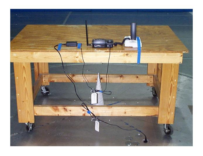
Figure 11-2: Configuration photograph, radiated emission, rear view
