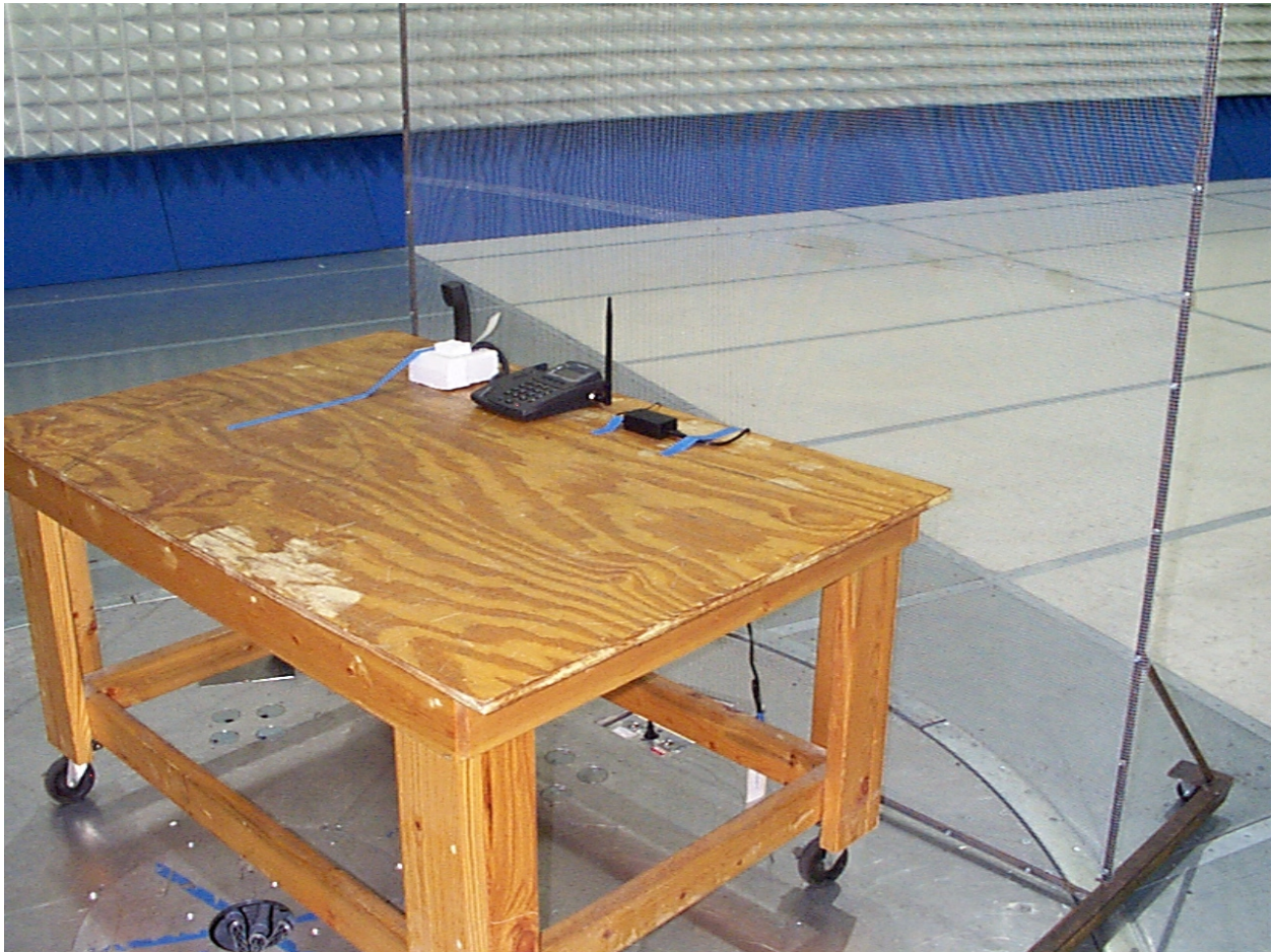
Figure 8-5: Configuration photograph, AC mains conducted emission, front view
