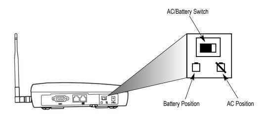
Figure 4 – SX5e AC/Battery switch.
