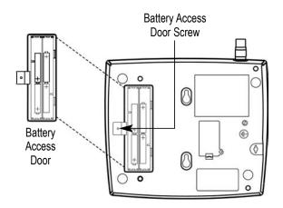
Figure 3 – SX5e battery installation.
