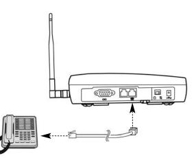
Figure 10 - Connect SX5e to Telephone.
