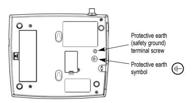
Figure 9a - Earth ground terminal screw.
