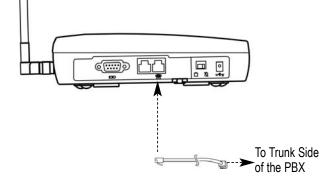
Figure 14 - Connect to trunk side of PBX.
