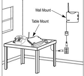
Figure 6 – Typical SX5e installation.
