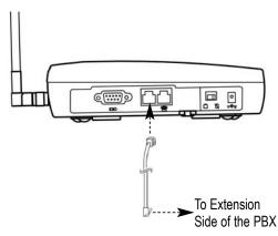
Figure 15 - Connect to extension side of PBX.
