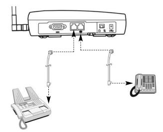
Figure 12 - Dual Jack mode connections.
