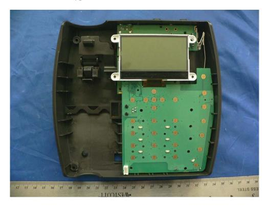
9.8 EUT – PCBA 1 Keyboard detail view side 1
