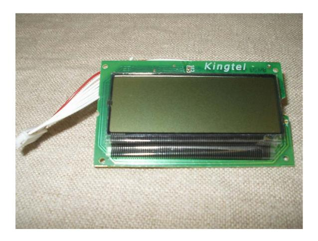
Figure 1-3: Internal photograph, LCD PCB (top)
