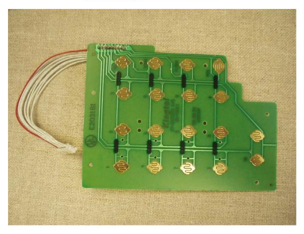
Figure 1-1: Internal photograph, Keypad PCB (top)
