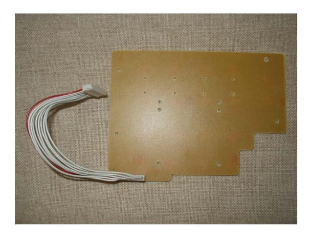
Figure 1-2: Internal photograph, Keypad PCB (bottom)
