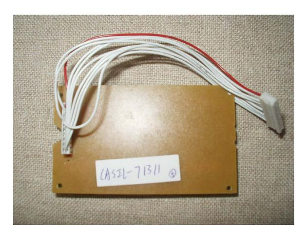
Figure 1-4: Internal photograph, LCD PCB (bottom)
