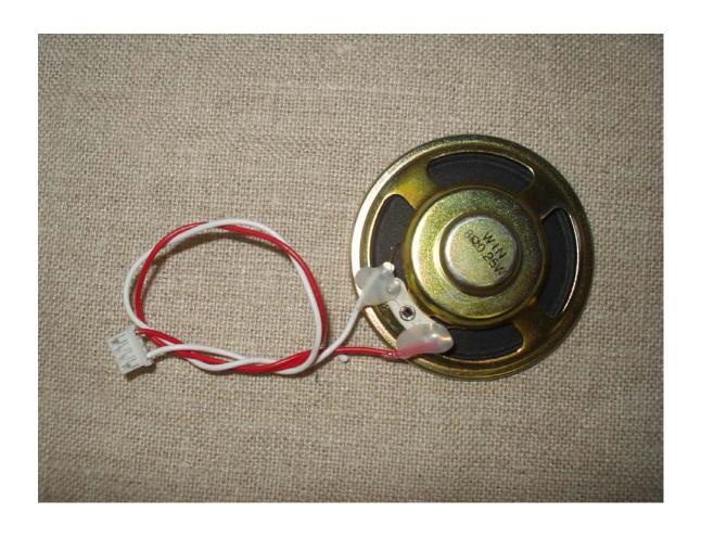
Figure 1-6: Internal photograph, speaker (back)
