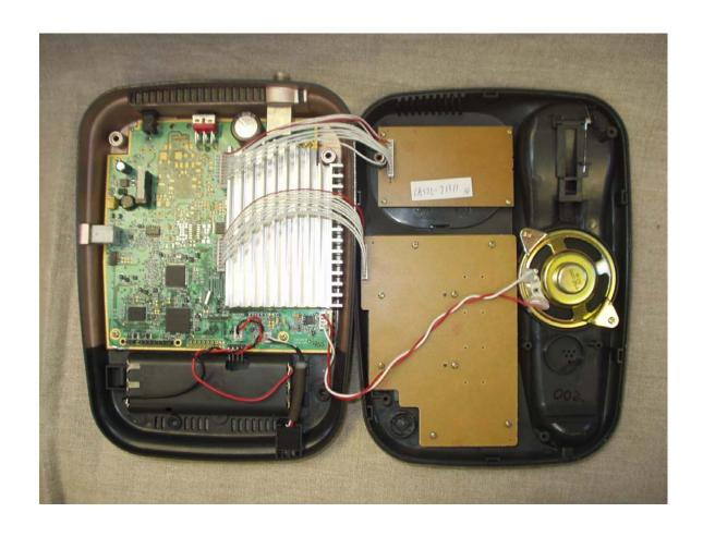
Figure 1-1: Internal photograph, SX4P enclosure with internal components
