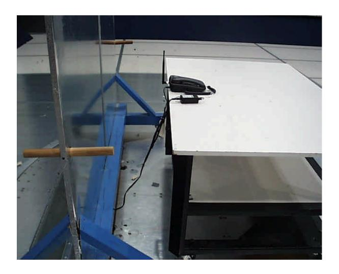
Figure 10-3: Configuration photograph, AC mains conducted emission, rear view
