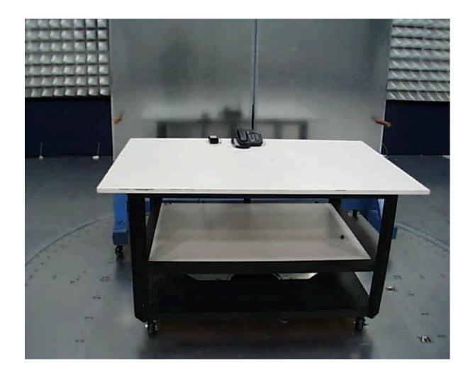
Figure 10-2: Configuration photograph, AC mains conducted emission, front view
