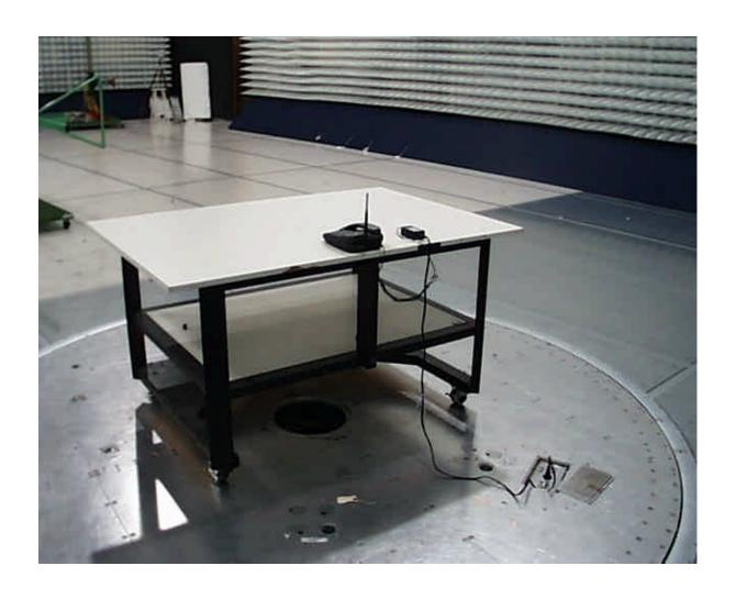
Figure 13-2: Configuration photograph, radiated emission, rear view
