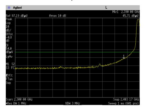
Restricted Band 2483.5 – 2500 MHz – Peak Tuned Freq = 2480 MHz
