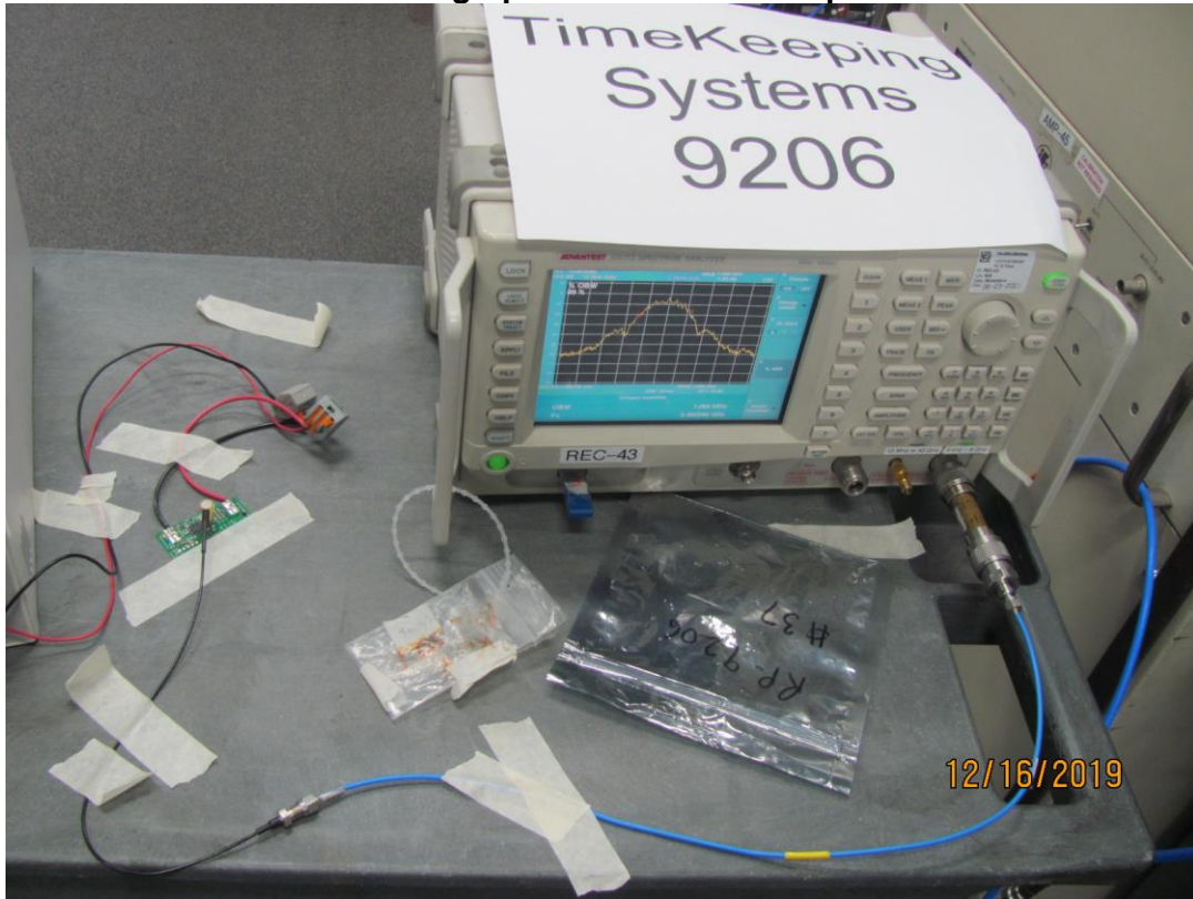
Photograph of OBW Test Setup
