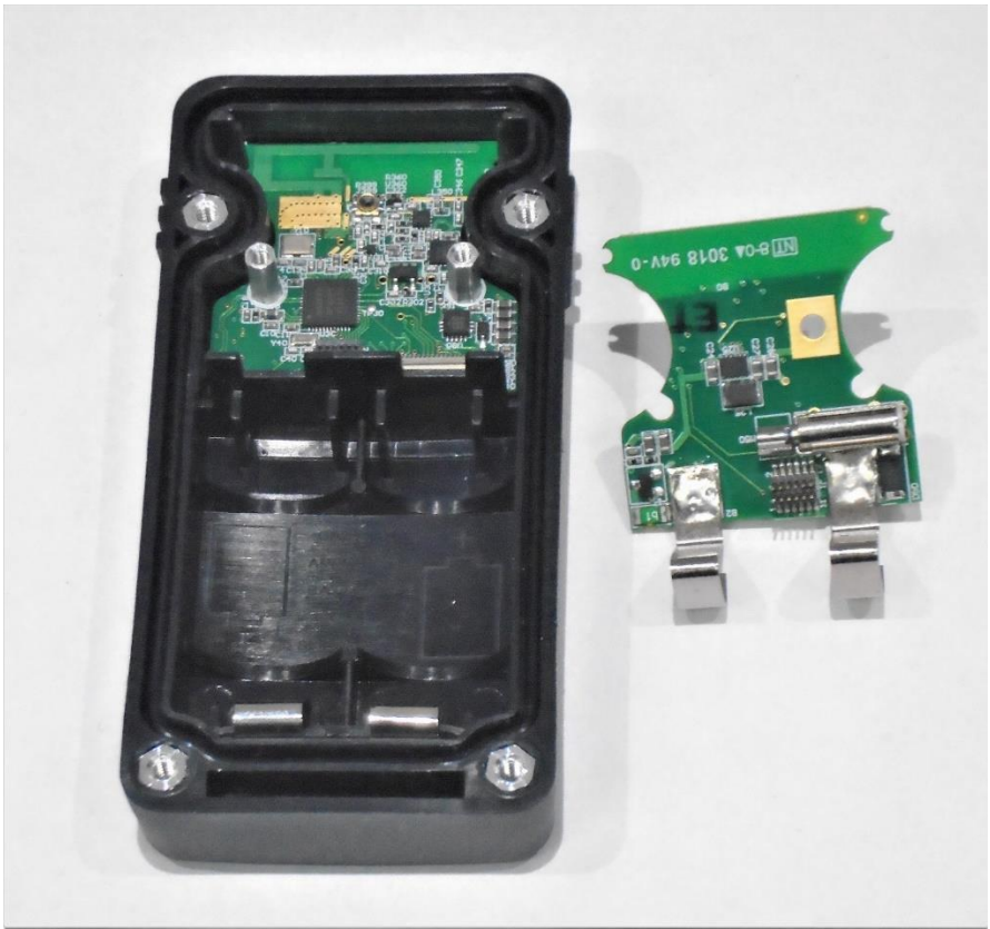
Interior with first PCB installed.
