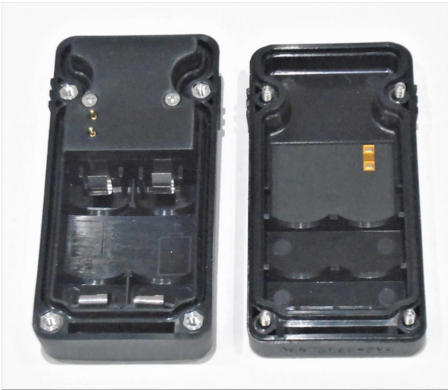
Interior with PCBs and inner PCB cover installed
