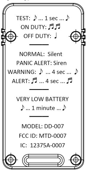
The label will be indelibly pad-printed directly onto the back of the plastic housing. The dimensions of the label are 1 1/8" wide by 3" tall
