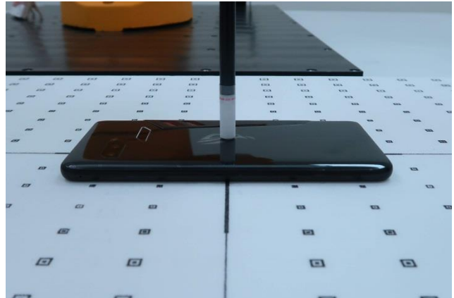
Front, Probe sensor to EUT surface distance 2mm Back, Probe sensor to EUT surface distance 2mm
