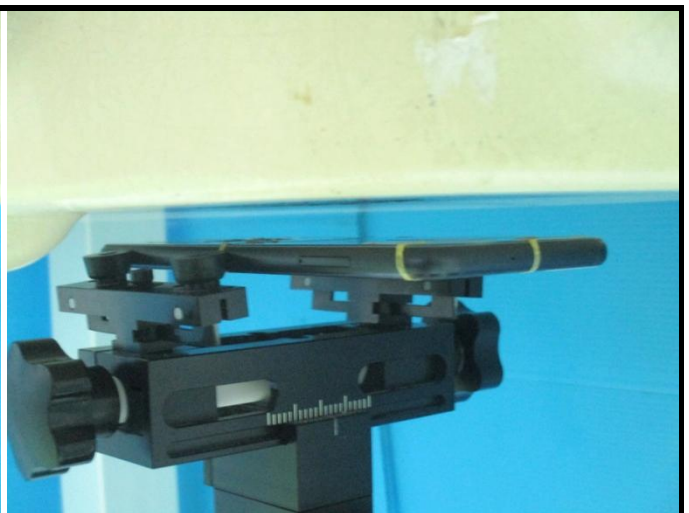
Hotspot - Rear Face of EUT at 10 mm
