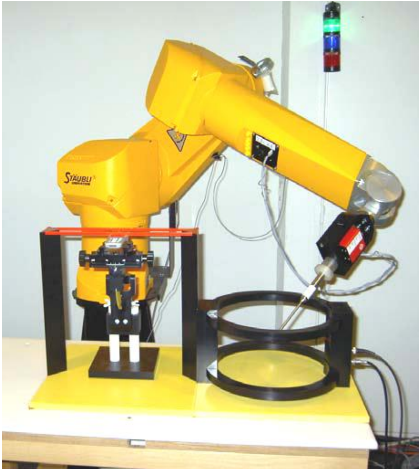
Fig. 5.1 T-Coil setup with HAC Test Arch and AMCC
