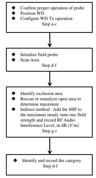
Fig 8.1 Flow Chart of HAC RF Emission
