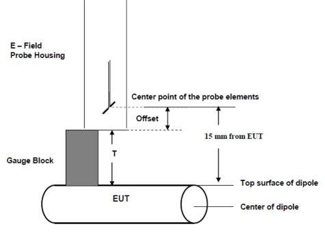
Fig. 8.3 Gauge block with E-field probe
