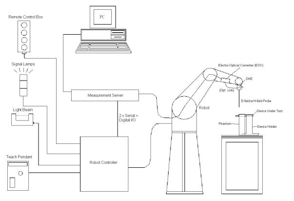
Fig 5.1 SPEAG DASY5 System Configurations
