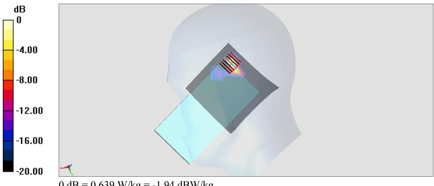
**#17\_WLAN5GHz\_802.11ac-VHT80 MCS0\_Right Cheek\_Ch155;Ant 2**
