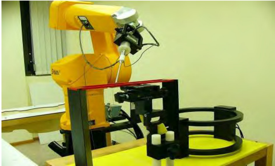
Fig. 1 Photograph of the DASY 5 measurement system
