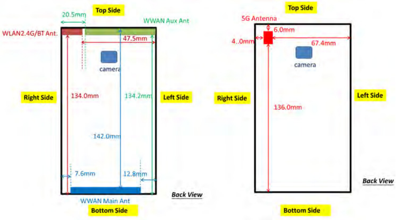
Fig.21 Antenna position of EUT
