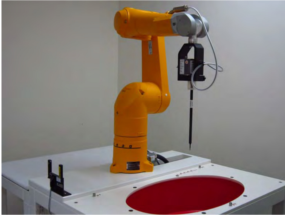
Fig.1 Photograph of the SAR measurement system
