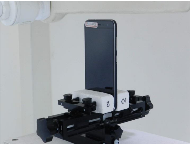
Top Side, Test Separation 10 mm
