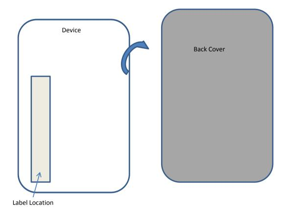
Label is visible to the users as they remove the back cover to install the SIM card.
