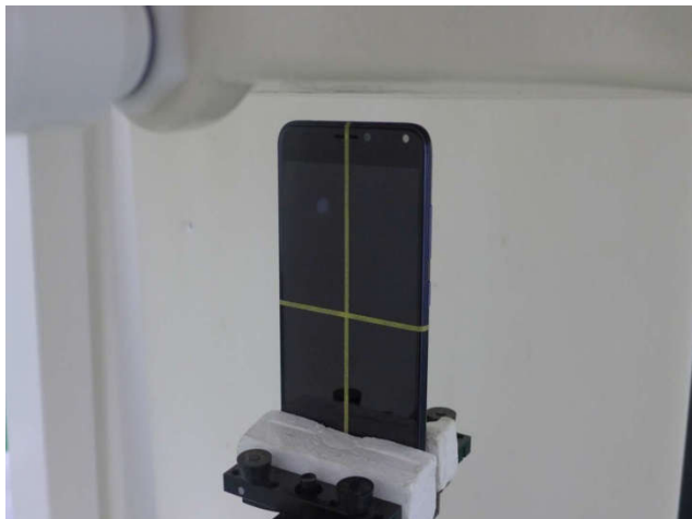
Top Side, Test Separation 10 mm
