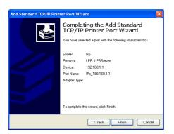
10. Install printer driver from the vendormodel list. If your printer is not in the list, click Have Disk to manually assign the location of driver.
