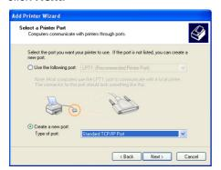
Input the IP address of WL-500gP in the Printer Name of IP Address field and click Next.
