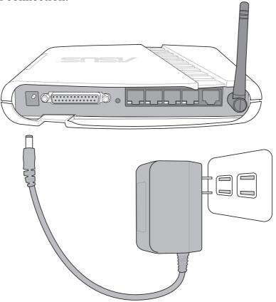
Note: Use the Home Gateway only with the power adapter supplied in the product package. Using another power supply may damage the Home Gateway.
