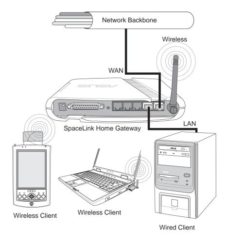
In this topology, the home gateway is an agent between your LAN and another network. Use a network cable with one end connected to the WAN port on the home gateway and the other to the other network as shown above.
