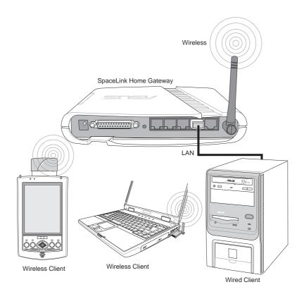
In this topology, the home gateway connects your wired and wireless devices together to form a local area network (LAN), as shown. To connect a computer (or other device) to the SpaceLink Home Gateway, you need a network cable (UTP-Cat5) with one end connected to one of the LAN ports on the back of the SpaceLink Home Gateway and the other in the 10/100 LAN port on that device. For wireless connections, wireless mobile clients must comply with the IEEE 802.11b standard.
