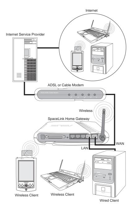
In this topology, the home gateway is not only a backbone of your LAN but also an agent to your Internet Service Provider (ISP). You may use an ADSL or Cable modem to communicate with your ISP. Connect the LAN port on the modem with the WAN port at the back of the SpaceLink Home Gateway using a network cable as shown above.
