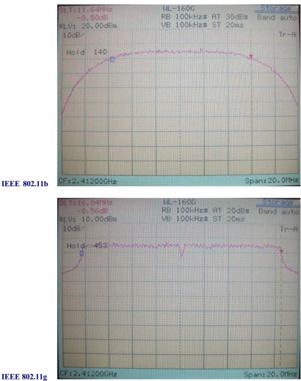
6dB Bandwidth of Channel 1 (The minimum 6dB BW at least 500kHz)
