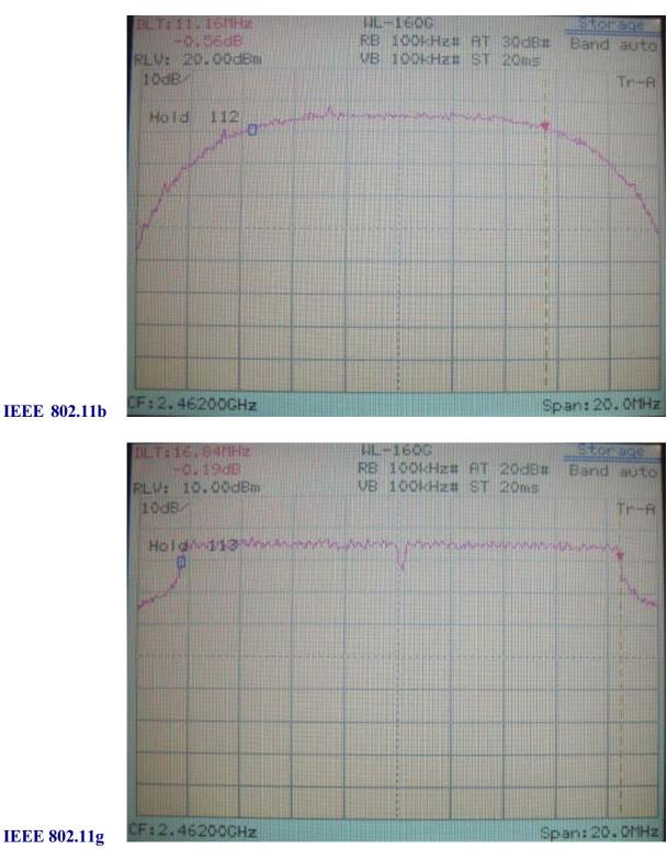
6dB Bandwidth of Channel 11 (The minimum 6dB BW at least 500kHz)
