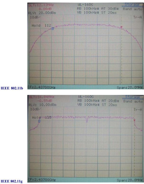
6dB Bandwidth of Channel 6 (The minimum 6dB BW at least 500kHz)
