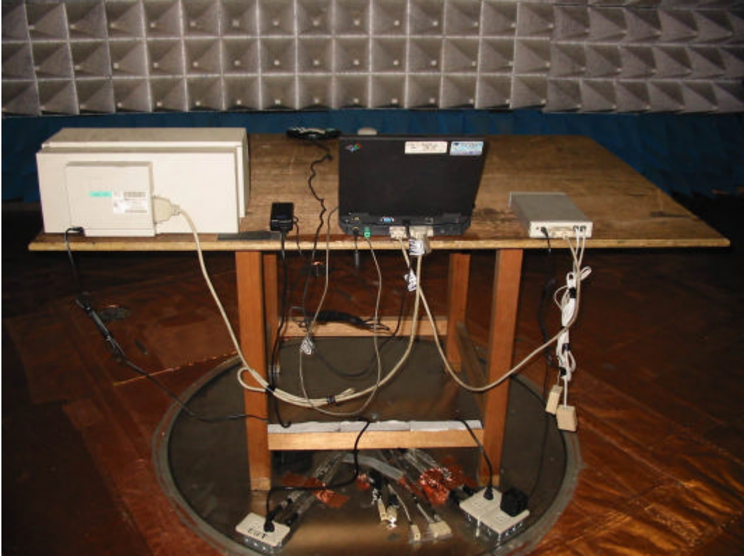
Rear View of the Test Configuration of Unintentional
