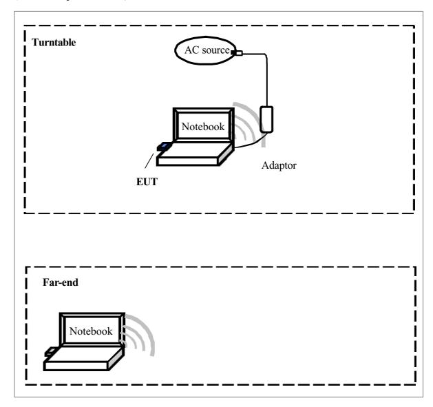
The tests below are carried with the EUT transmitter set at high power in TDD mode. The EUT is forced to select of output power level and channel number by notebook computer.
