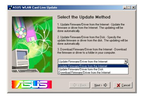
**Update Firmware/Driver from the Internet:** Lets you update the ASUS SpaceLink PC Card's firmware or driver from the Internet. The updating (running the flash utility or the installation program) will be done automatically.
