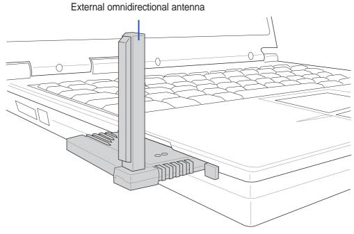
Inserted ASUS SpaceLink PC Card - Antenna Up
