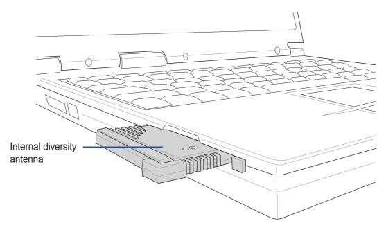
Inserted ASUS SpaceLink PC Card - Antenna Down
