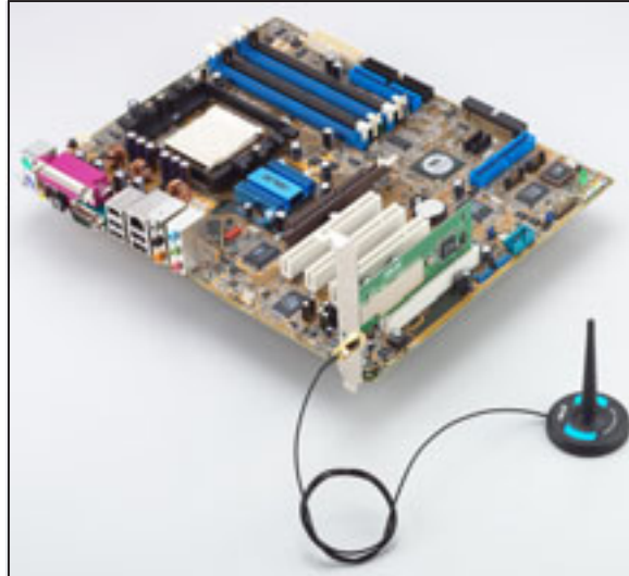
A WiFi-g™ card installed to an ASUS motherboard
