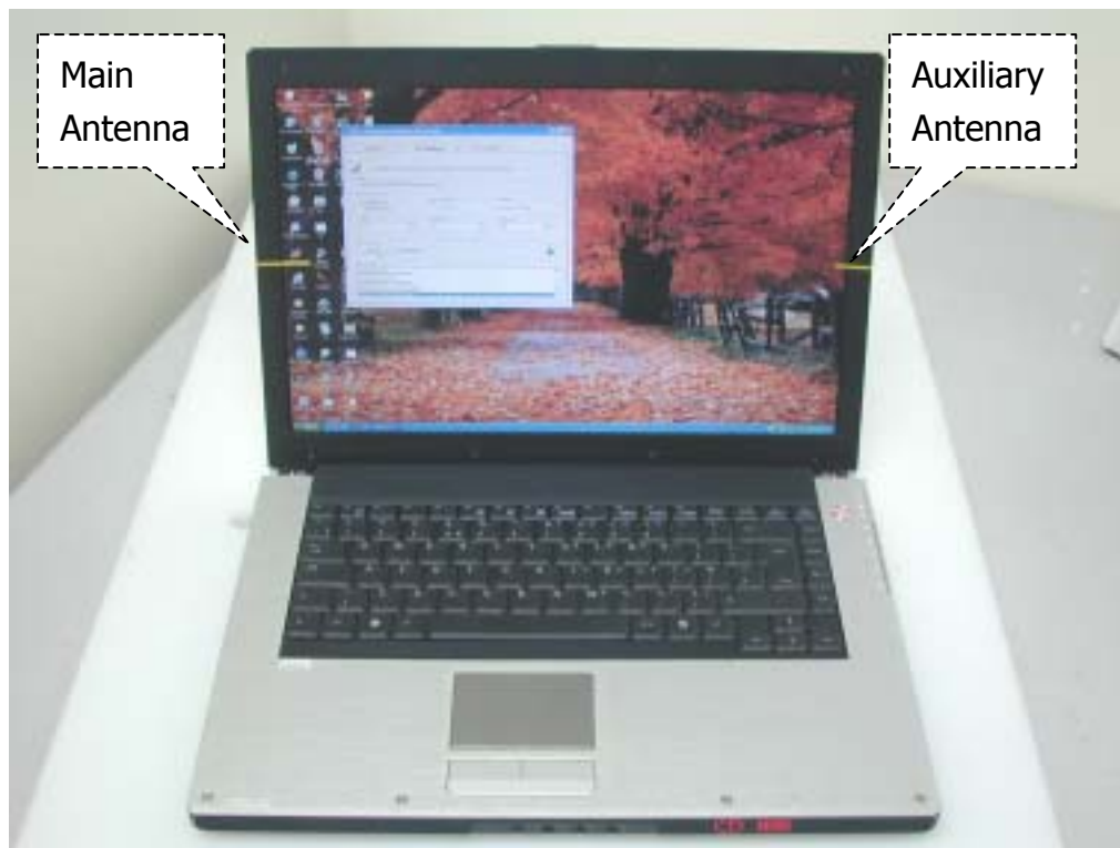
Fig.9 Antenna Position of EUT
