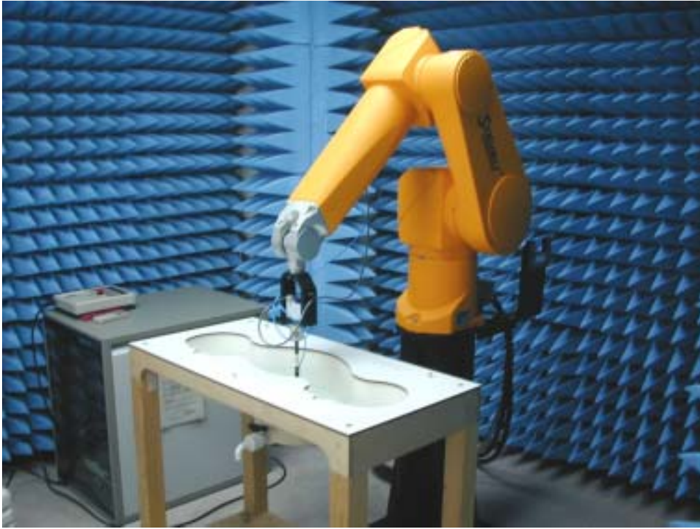
Fig.1 Photograph of the SAR measurement System
