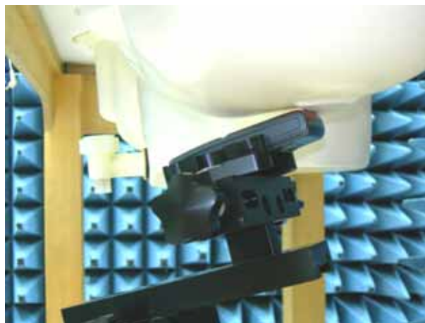
Figure 13. Left Head SAR Test Setup (Tilted)
