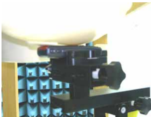
Figure 14. Right Head SAR Test Setup (Cheek)
