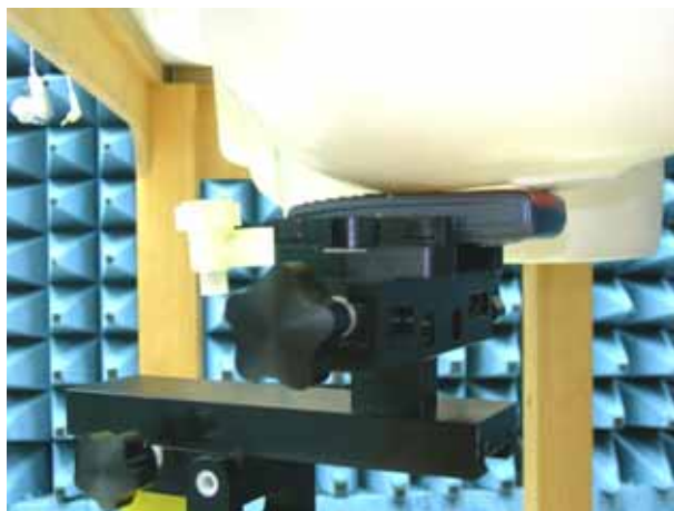
Figure 12. Left Head SAR Test Setup (Cheek)
