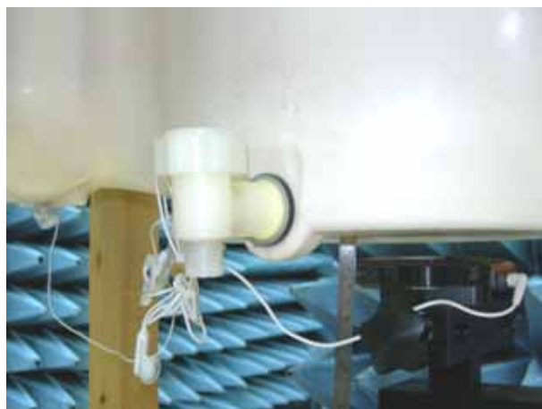
Figure 16. Body SAR Test Setup (Flat Section)
