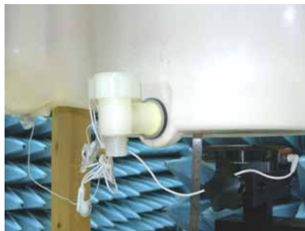
Figure 17. Body SAR Test Setup (Flat Section)
