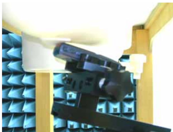
Figure 15. Right Head SAR Test Setup (Tilted)
