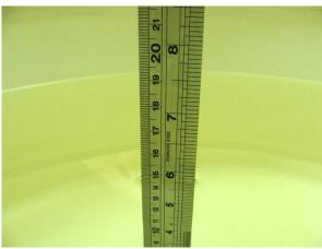
Fig 6.1 Photo of Liquid Height for Head SAR
