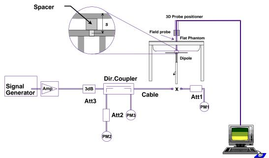
Fig 8.1 System Setup for System Evaluation
