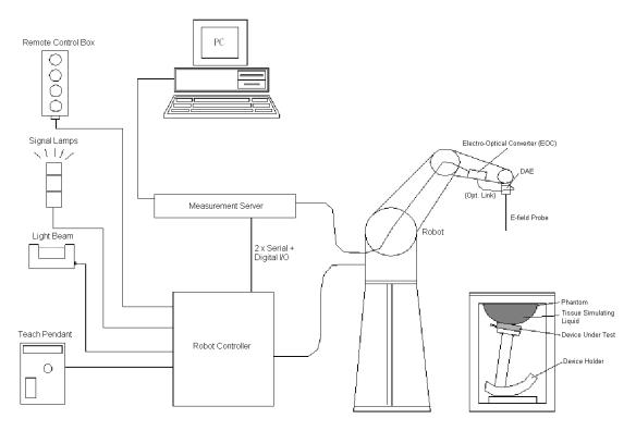
Fig 5.1 SPEAG DASY5 System Configurations
