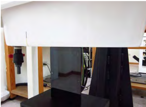
Fig.5 EUT Primary Portrait mode to flat phantom (Test distance is 0 mm)
