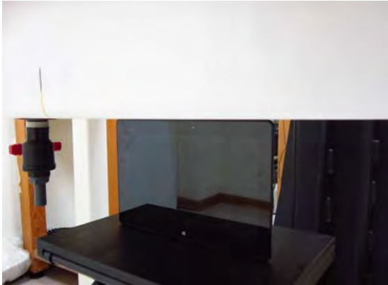
Fig.6 EUT Secondary Landscape mode to flat phantom (Test distance is 0 mm)
