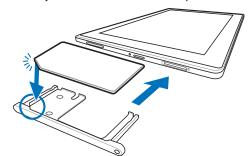
3. Firmly push the SIM card tray back to the slot.
