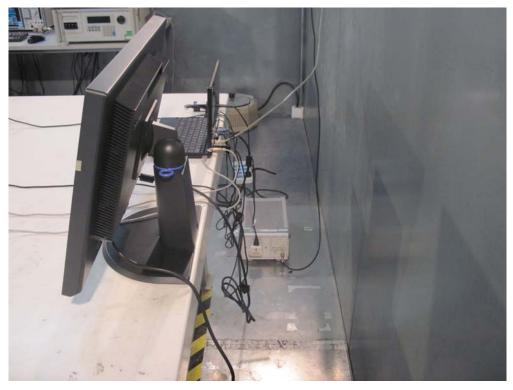
Test Mode : Transmitting Description : Front View of Radiated Emission Test Setup for Below 1GHz
