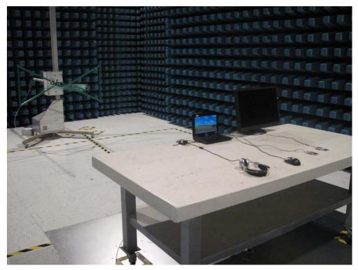
Test Mode : Transmitting Description : Front View of Radiated Emission Test Setup for Above 1GHz
