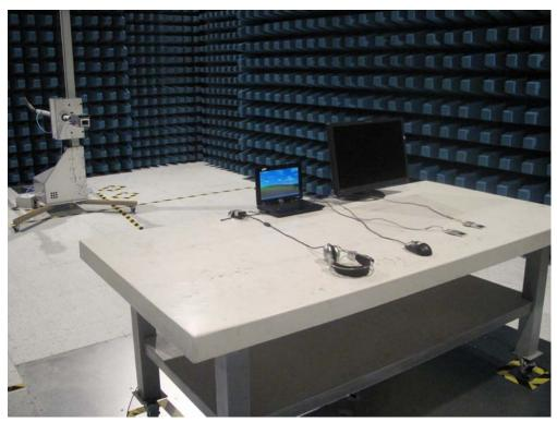
SAR Test setup
