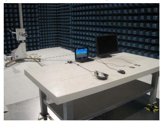
**SAR Test setup**
