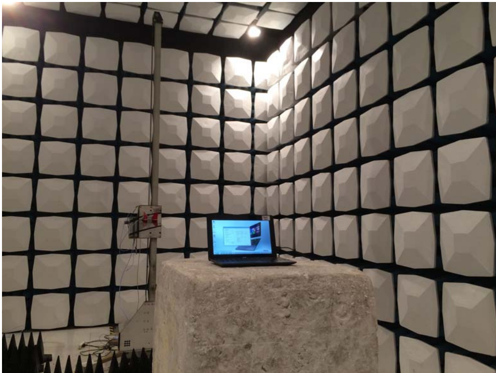
Description: Radiated Emission Test Setup for 1~18GHz
