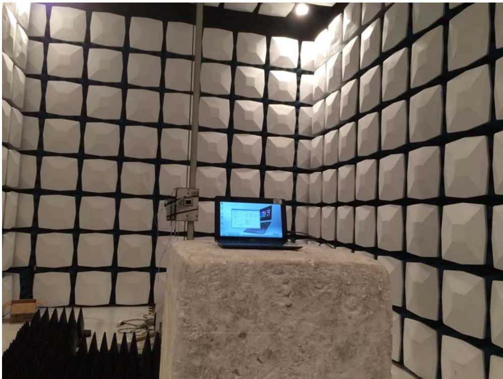
Description: Radiated Emission Test Setup for 18~40GHz
