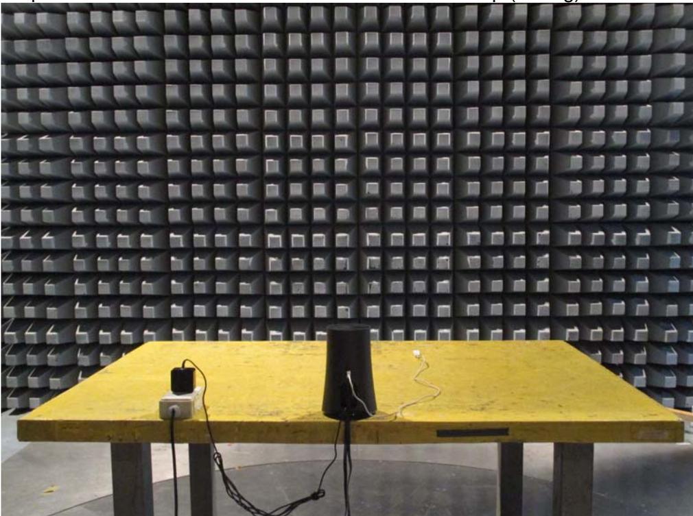
Test Mode : Mode 6: Tx- Vertical Antenna (ADP-33AW)
