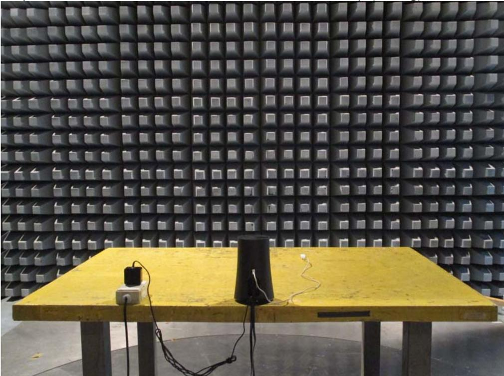
Test Mode : Mode 1: Tx- Horizontal Antenna (AD891M21)
